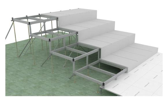
FLOOR and more<sup>®</sup> arena Substructure with planking whose base is connected to a FLOOR and more<sup>®</sup> system.
